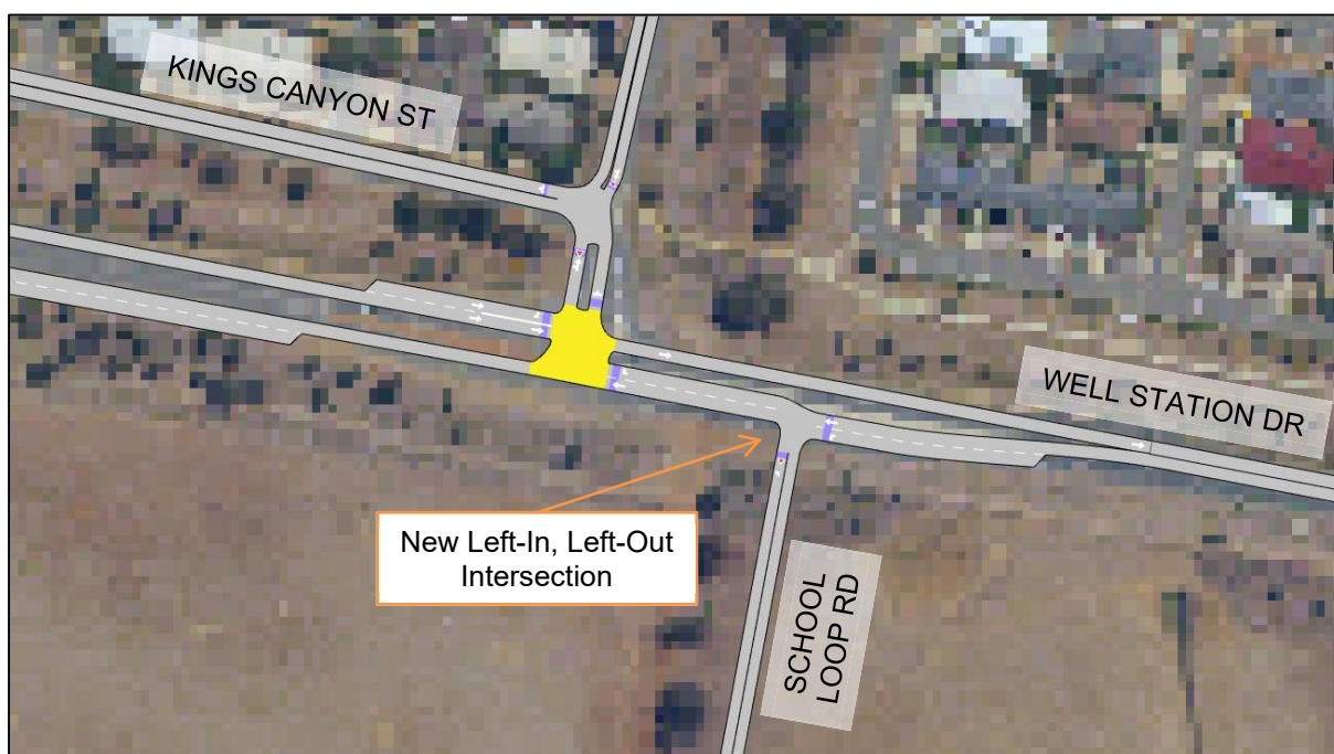
Figure 14. Works Package L – School Loop Road / Well Station Drive: Left-In, Left-Out Access
