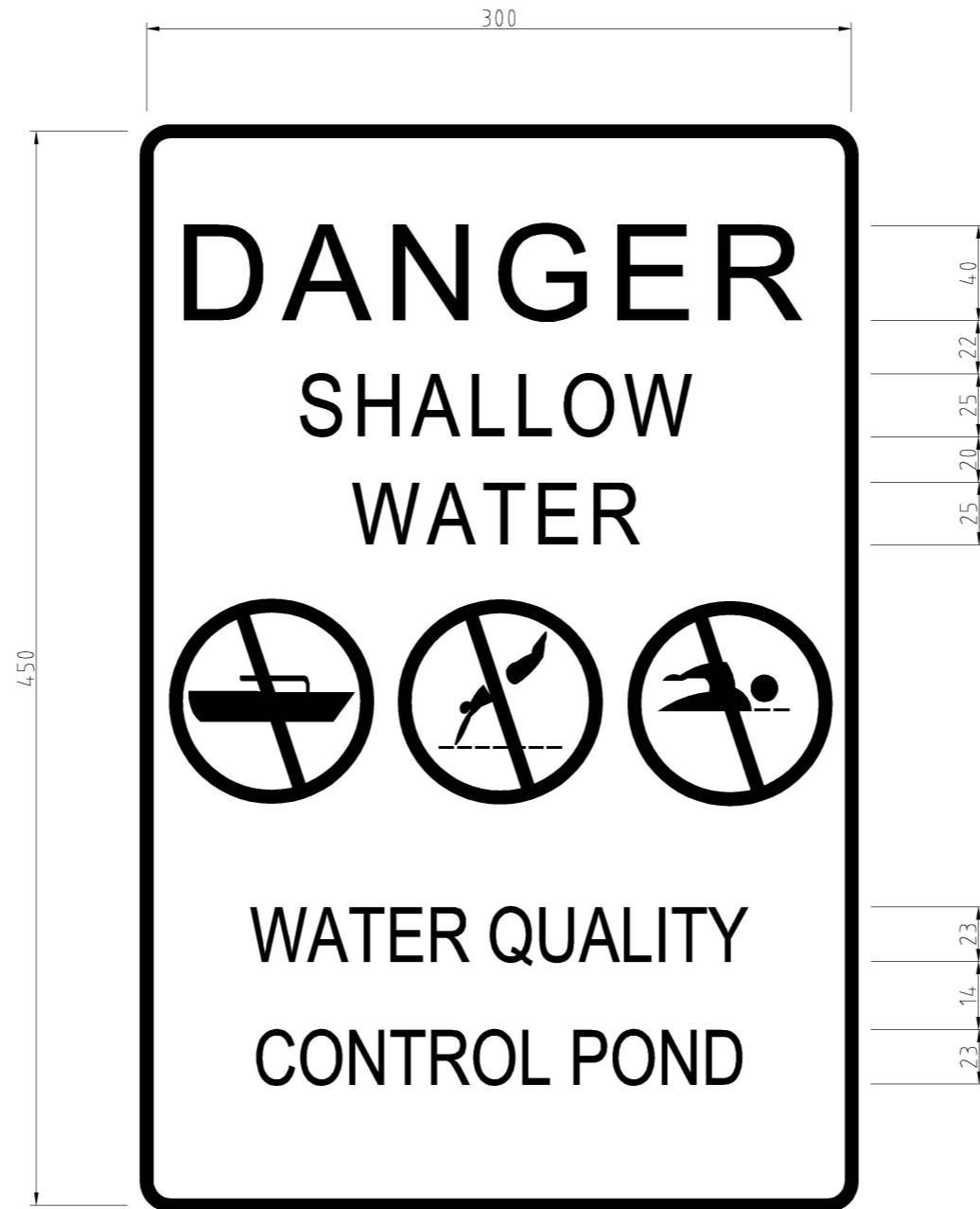
WATER QUALITY CONTROL POND WARNING SIGN
