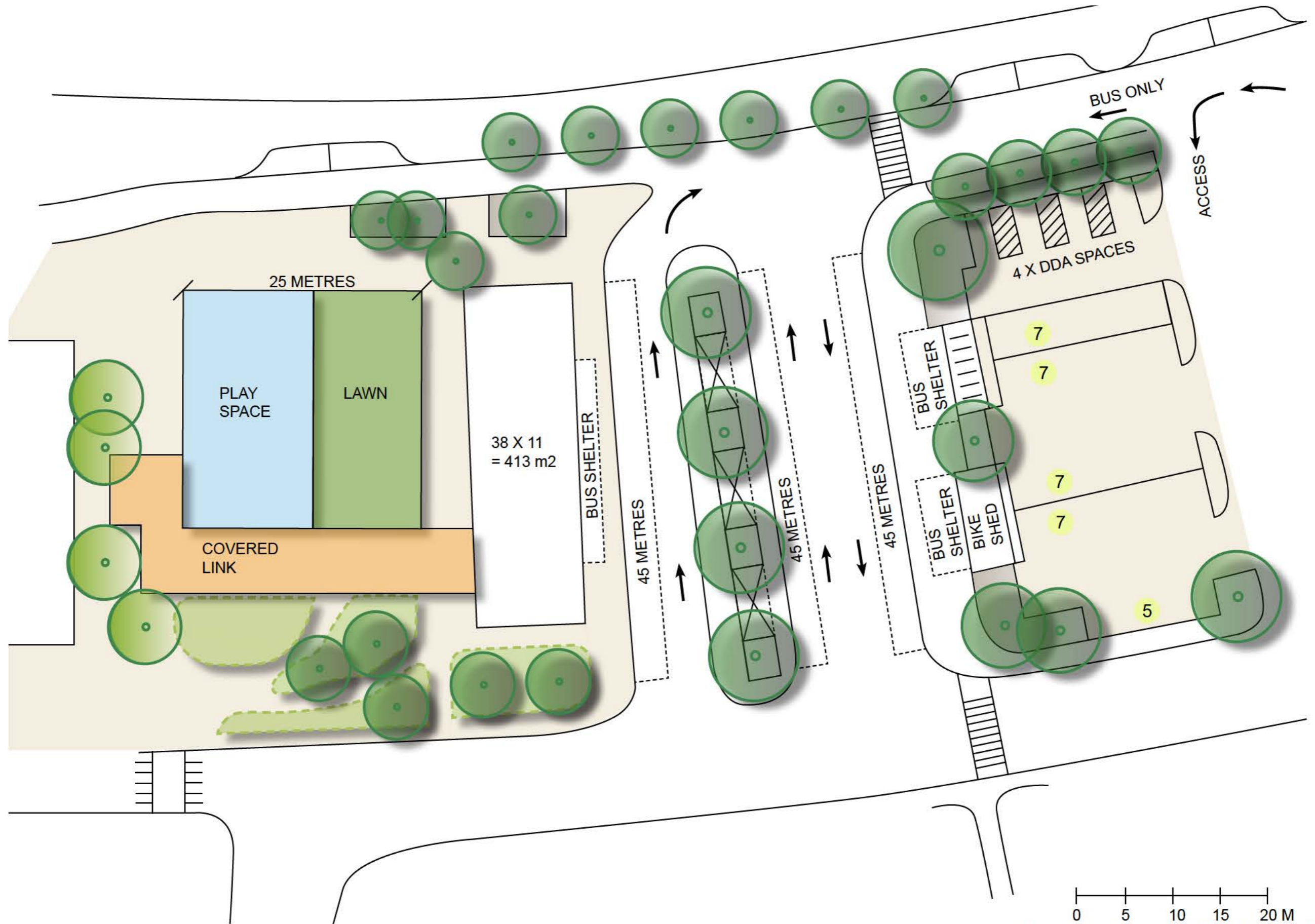
Figure 16. Bus Interchange Additional Platform Option
