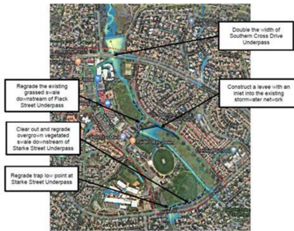
Figure 1-2: Recommended Mitigation Measures to Alleviate Existing Flooding
