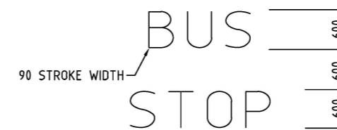
USE SAME SPACING FOR KEEP CLEAR TYPICAL PAVEMENT LETTERING CAD CODE: BUSSTOP
