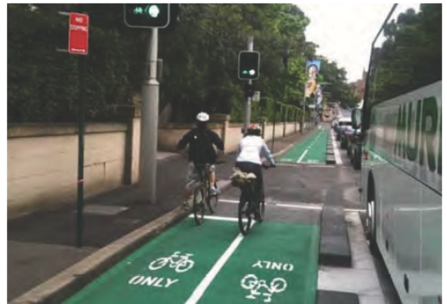
Separated Cycleways: Raised median
