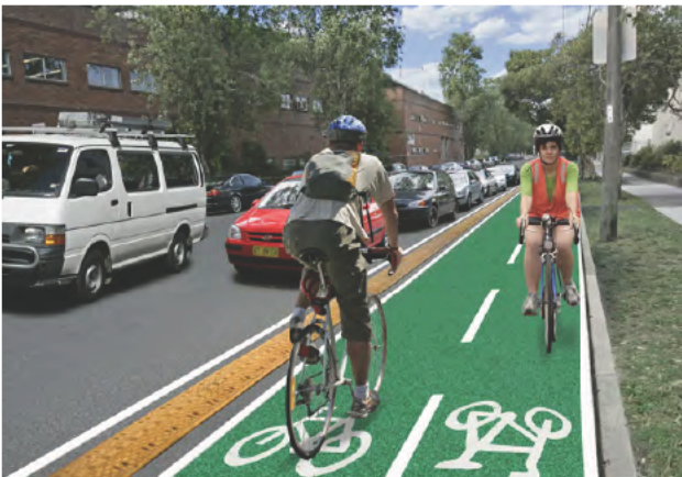
Separated Cycleways: Surface mount lane dividers
