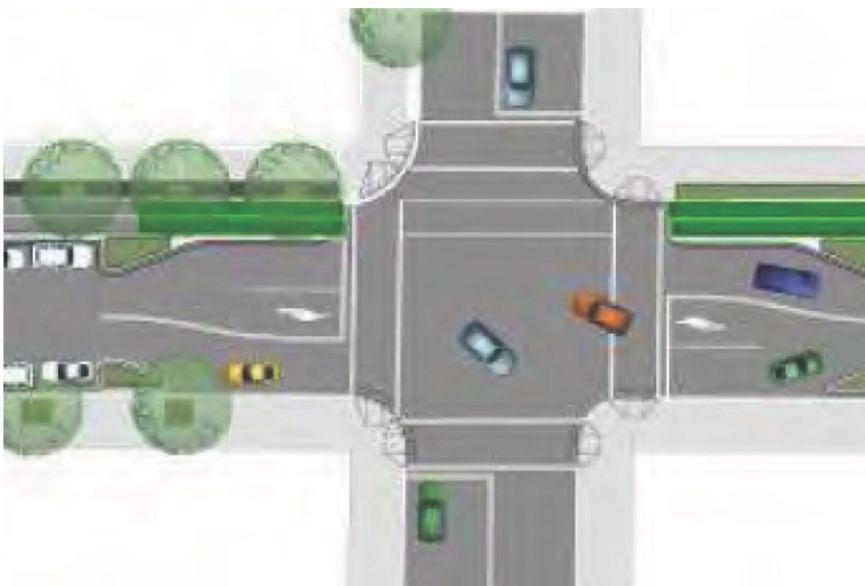
Signalised Intersection, Typical plan (City of Sydney)
