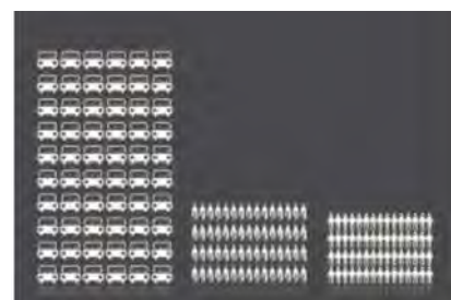
Comparison of space utilisation of 60 cars, cyclists and people from the National Cycling Strategy
