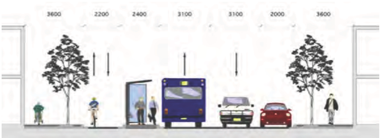
Section showing a typical treatment at bus stops along cycleways (City of Sydney)
