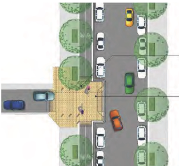
Shared Environ Intersection, Typical plan (City of Sydney)
