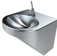
Single stainless-steel wall-mounted vanity basins with integral shroud - easier to clean and more secure than those with exposed pipework. Vanity Basins should only be used when integrated with stainless steel bench top. Note robust stainless-steel tap with timed flow valves to avoid water wastage.
