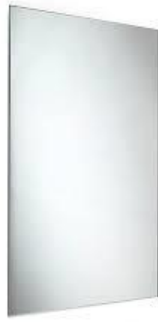
Stainless steel mirror. Refer AS1428.1 for minimum sizes and mounting heights. In all cases to be mounted directly above basin lip / splashback.
