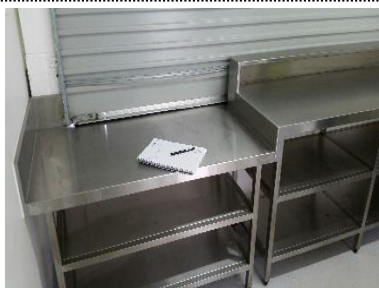
Stainless steel Food Servery bench with under shelving and splashbacks – two levels, one for children and typical for adult participants.
