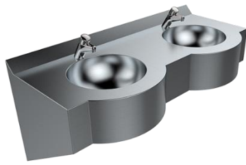
Multiple stainless-steel wall-mounted vanity basins with integral shroud - easier to clean and more secure than those with exposed pipework.
