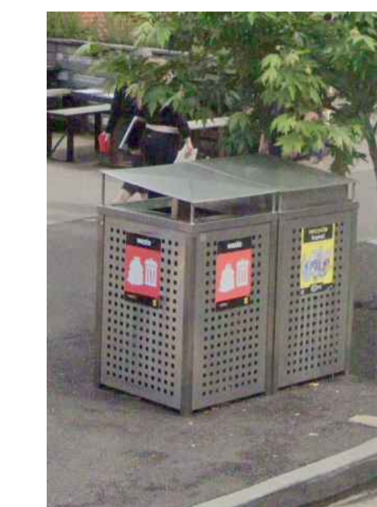
Supply + install twin bin surround Surface fix to new concrete slab 50mm wider all round x 100mm deep to 25 MPa
