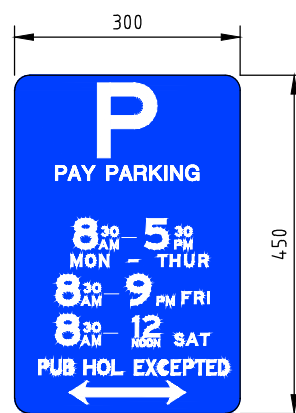
EXAMPLE AISLE/ON-STREET SIGN
