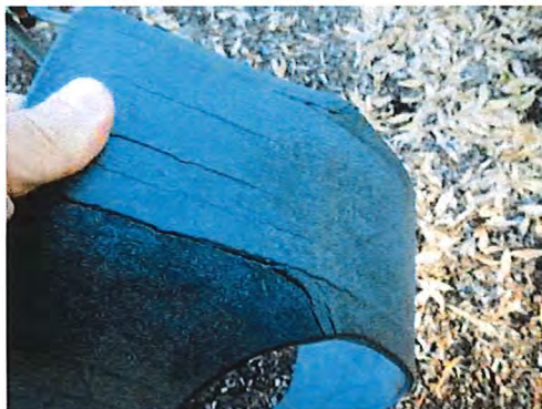
Photo taken: 25/05/2017 Toddler seat cracking. Monitor.
