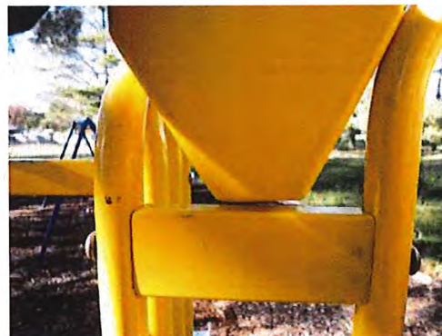
Photo taken: 13/05/2010 Neck probe just not touching the bottom
