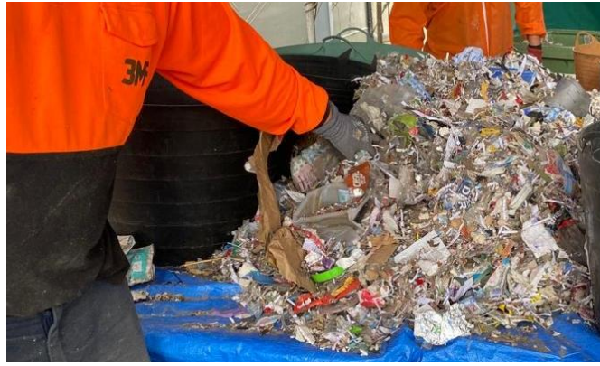
Image 14:: Residual fines – light, fluffy material with small quantities of dirt and glass sand
