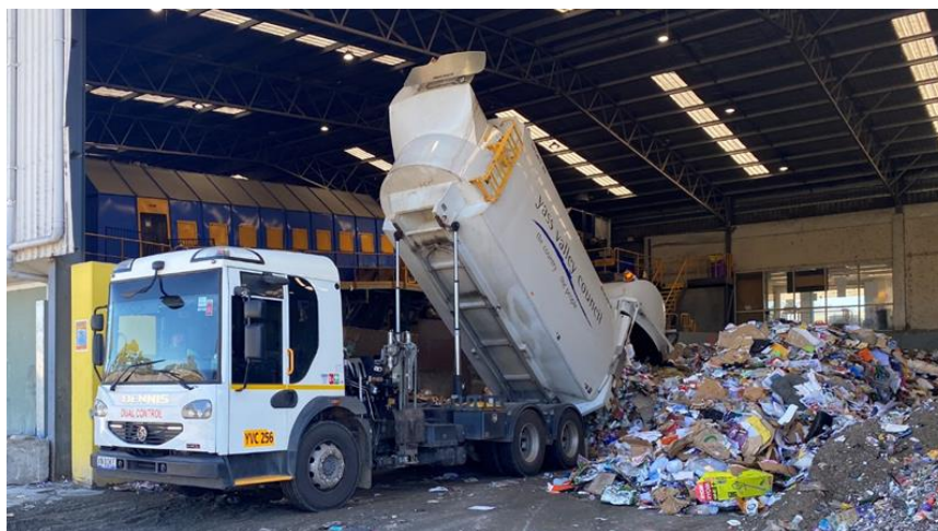
Image 2: Incoming kerbside loads depositing comingled recyclables at the feedstock hall
