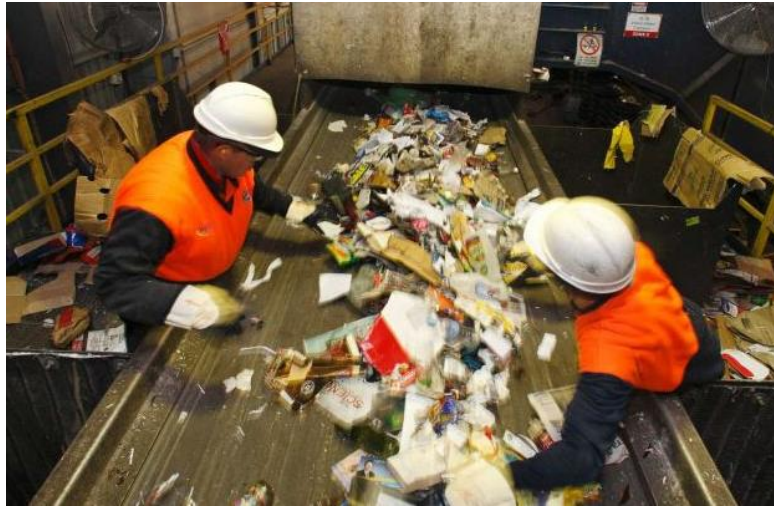
Image 3: Handpicking oversize, long, stringy or bagged material at the pre-sort station
