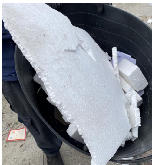
Image 20: Styrofoam (EPS) contamination in the RDOC sample
