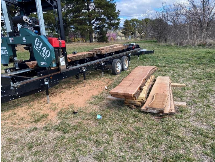
Image 10 Sawn timber produced from the portable mill
