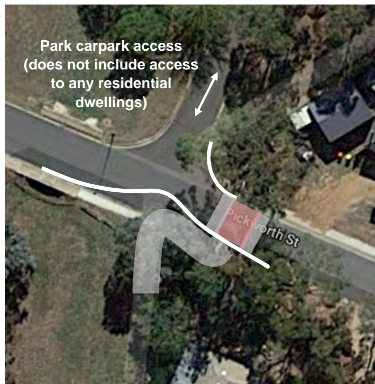
Figure 4 – Possible Pickworth Street crossing blister concept
