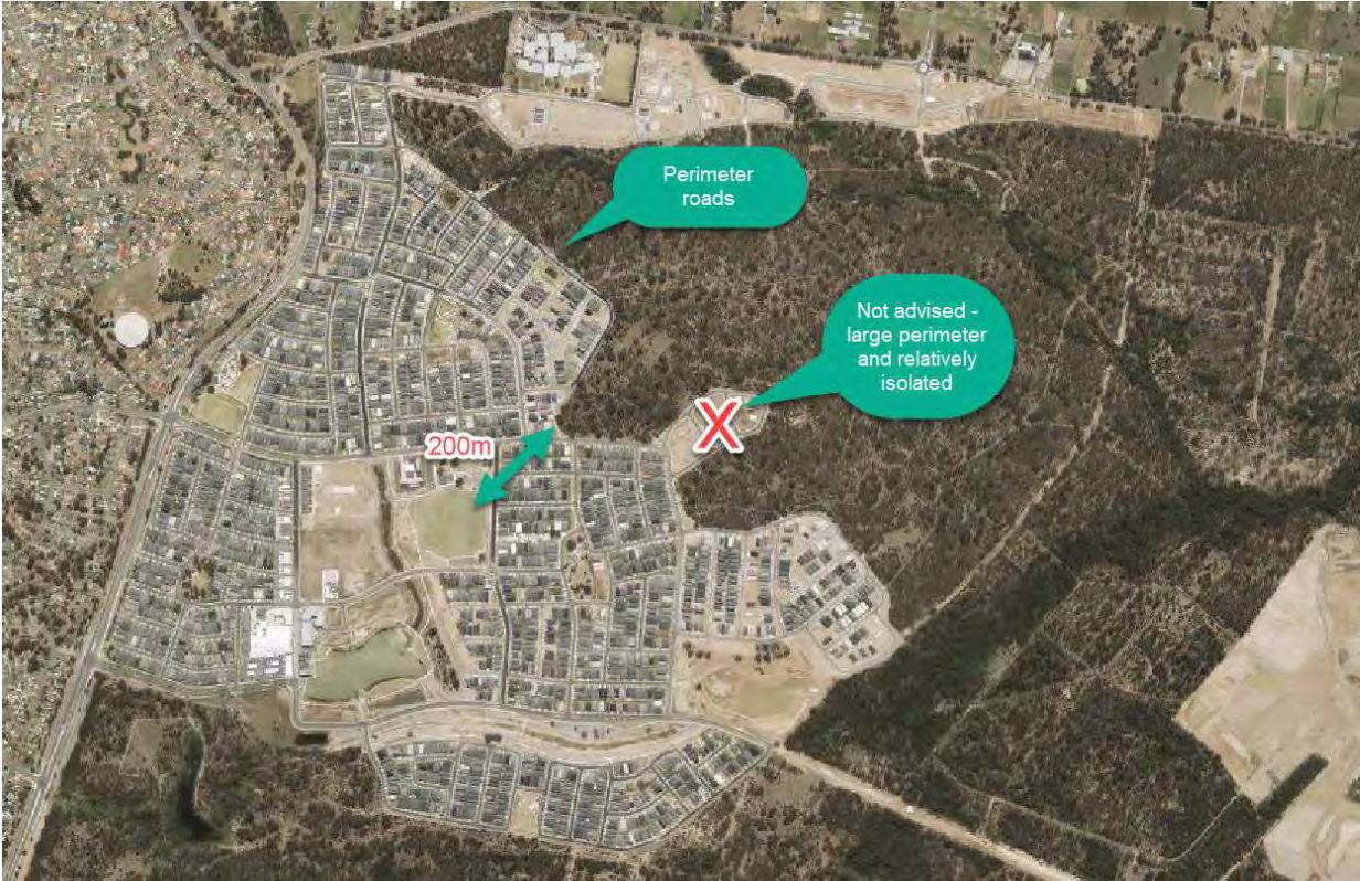
Figure 15: Planned interface with perimeter roads and access into large urban area - less chance of spread and lower impact likely.
