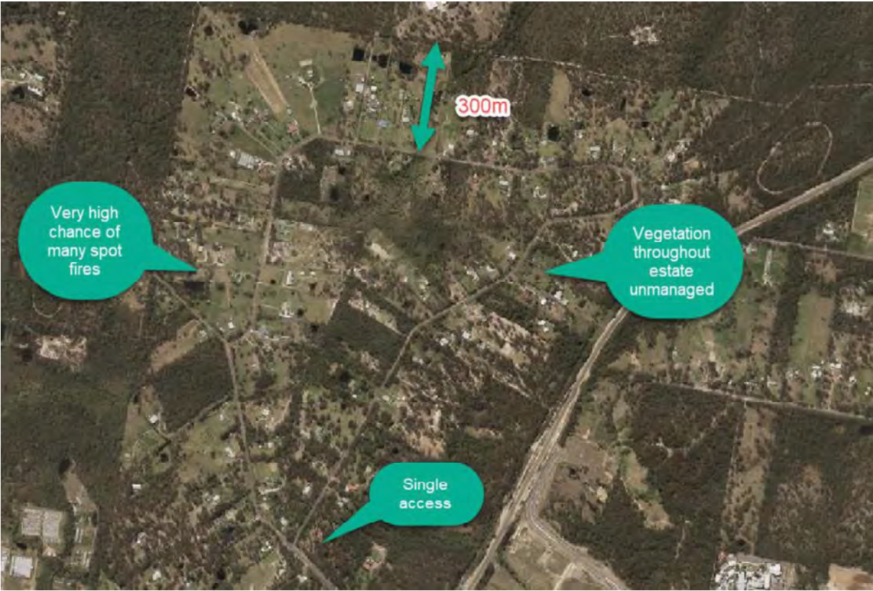
Figure 14: Dangerous intermix type development - rapid fire spread and large impact likely.
