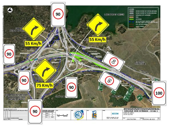
Figure 2 Suggested Speed Limits Glenloch Interchange
