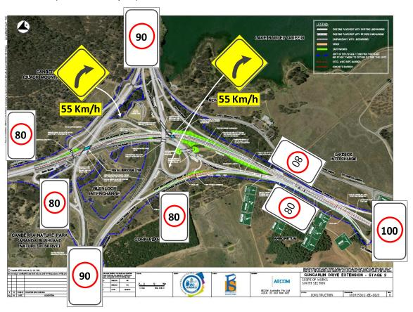
Figure 1 Existing Speed Limits Glenloch Interchange
