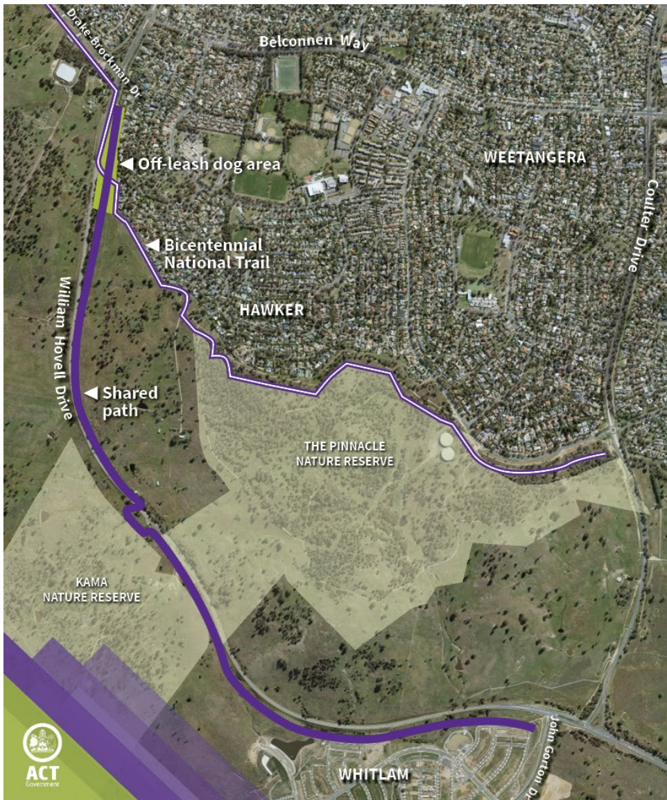
Image 2 – Map 2 – Shared path alignment along William Hovell Drive between Drake-Brockman Drive and John Gorton Drive.
