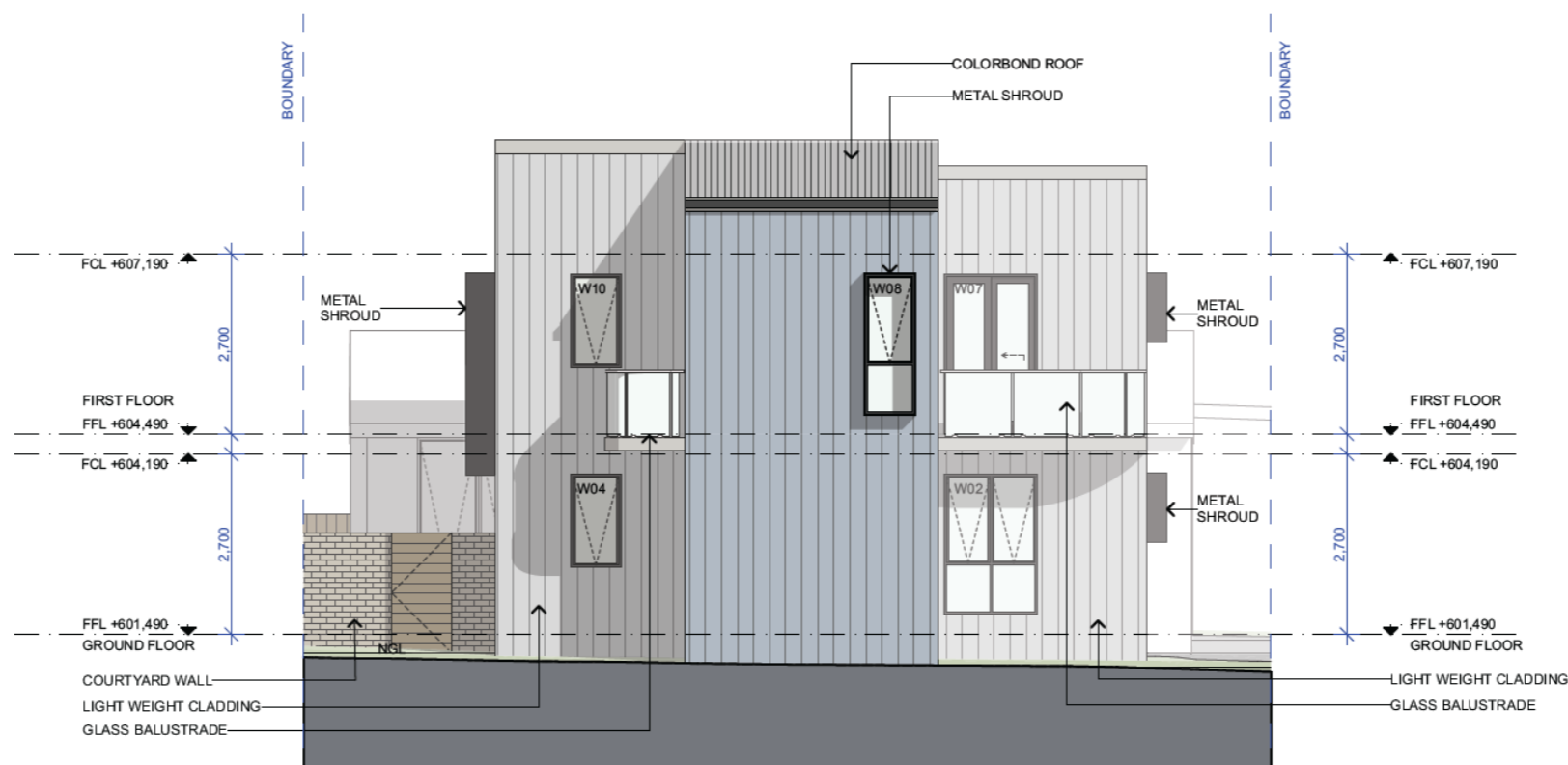
NORTH WEST ELEVATION
