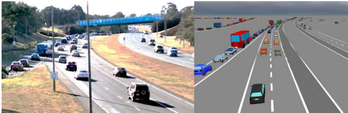
Figure 10 Cotter Road on-ramp – Observed vs model queues
