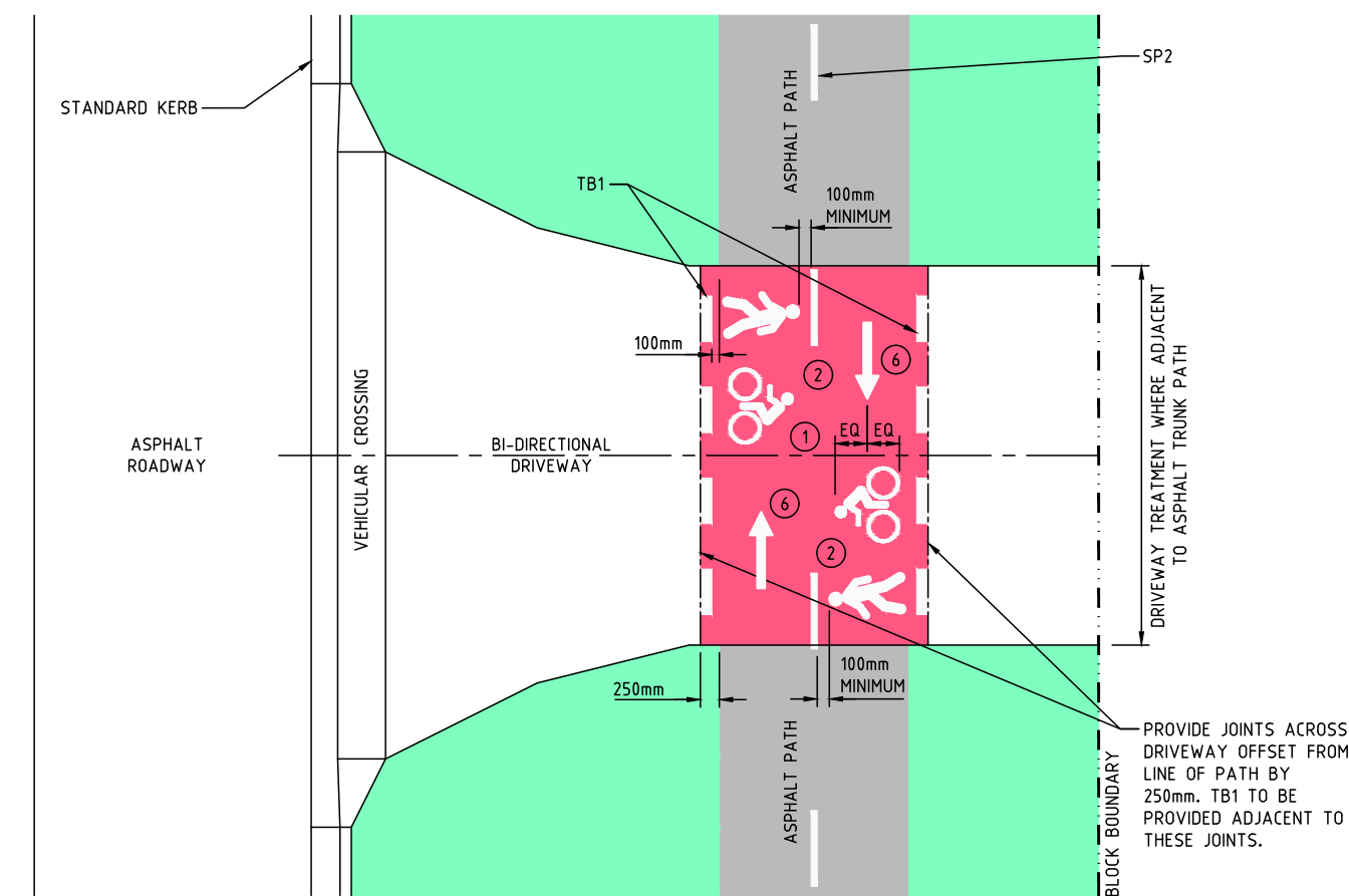
DRIVEWAYS TO MORE THAN 15 CAR PARKING SPACES MAIN OR LOCAL COMMUNITY ROUTE CROSSING OF DRIVEWAYS TO COMMERCIAL OR MULTI-RESIDENTIAL DWELLING SITES RETROFIT ONLY ⑧
