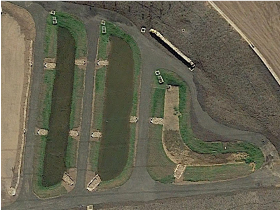
Figure 8-28 Cellular bioretention basin (Blacktown City Council)
