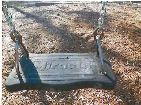
Photo taken: 24/05/2016 Bent suspension mounts.
