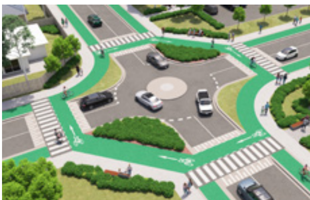
Aerial view of a traffic intersection model showing tightened kerb limits which slows turning traffic and increases visibility between road and path users.
