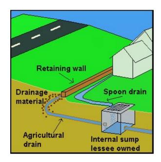
**Intercept** any seepage paths from springs, etc, by using free-draining gravels, agricultural drains and spoon drains.
