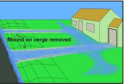
**Ensure** that the builder does not reduce the steepness of your driveway by removing the mound of soil between the gutter and boundary.
