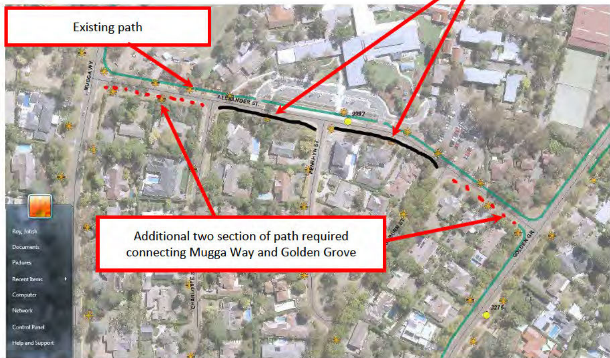
Figure 7: Proposed community path improvement in RED DOTTED LINES, Current community paths in SOLID BLUE LINES (based on GIS asset information)
