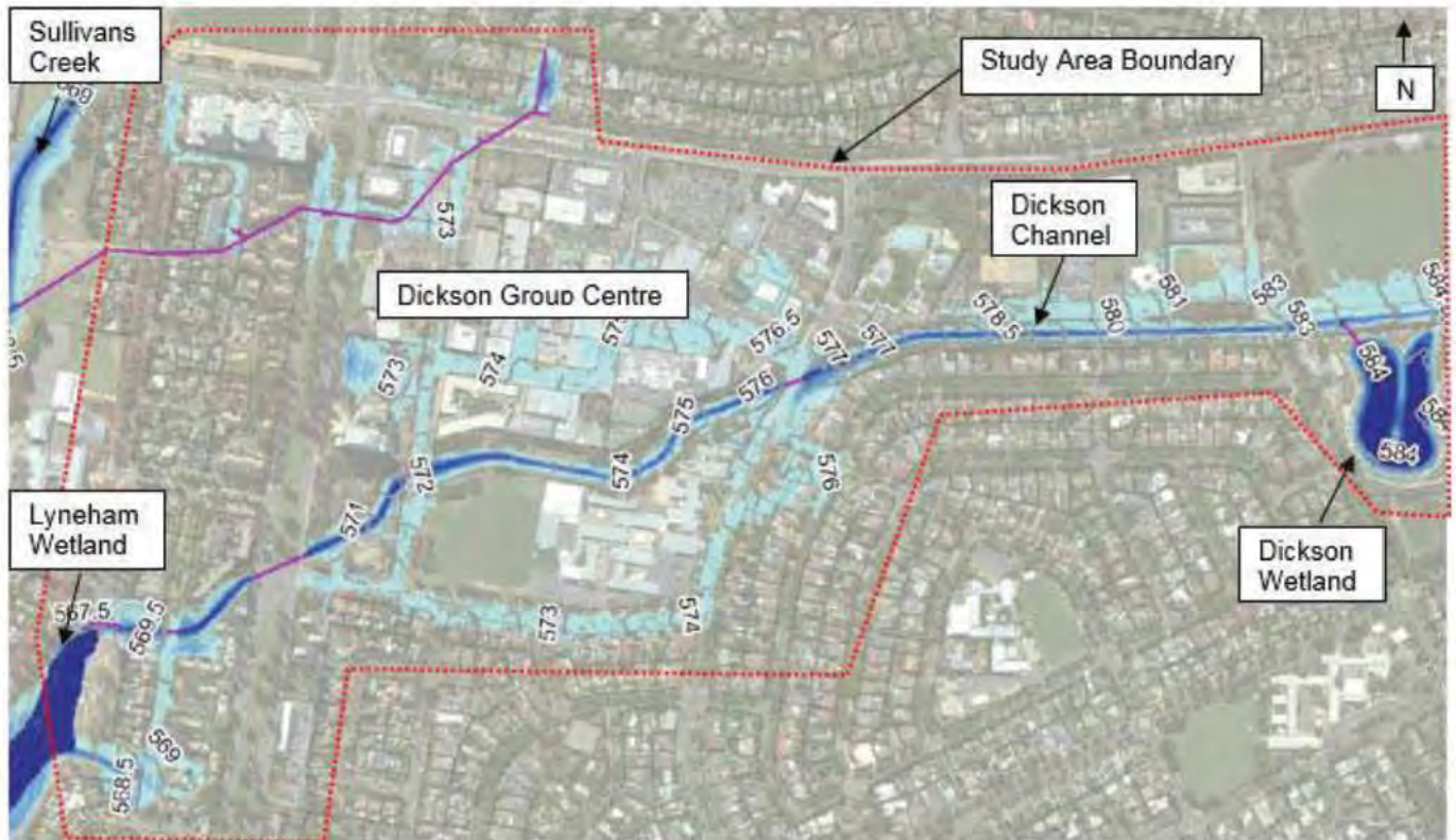
Figure 4-1: Study Area and existing 1% AEP flood extents
